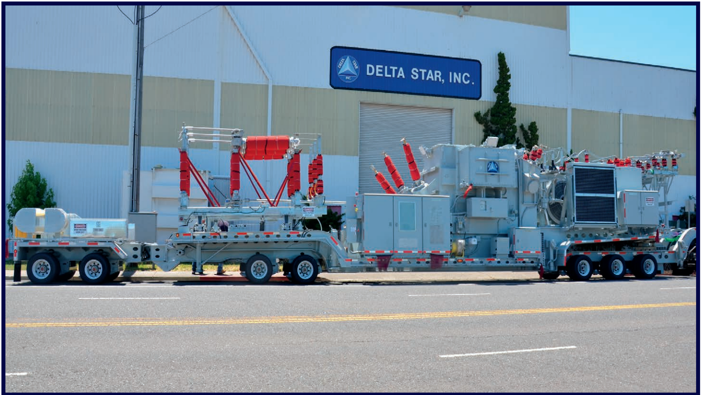
(35 MVA, 115 kV - 13.09 kV, LTC) 2017 | 82'-7" | 151,000 lbs. Customer Region: SOUTHEAST
