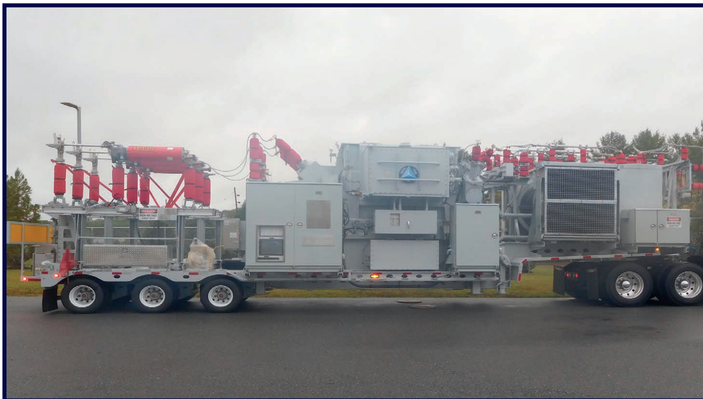
(25 MVA, 69 kV - 26.4 kV, LTC) 2017 | 54' | 124,000 lbs. LV Vacuum Breaker and HV Circuit Switcher Customer Region: MIDWEST
