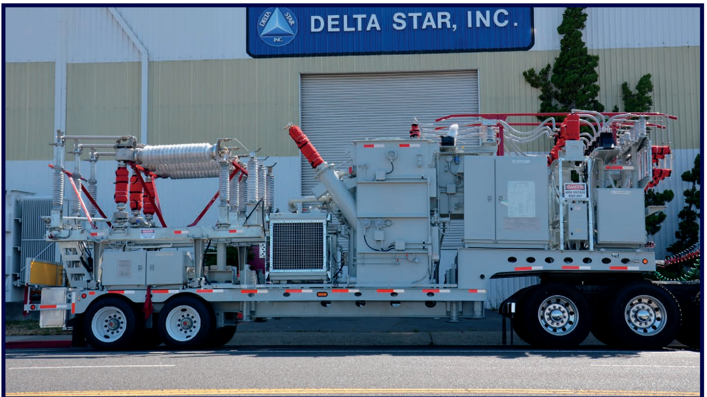
(10 MVA, 69 kV - 13.09 kV, LTC) 2015 | 32' | 89,000 lbs. Customer Region: MIDWEST
