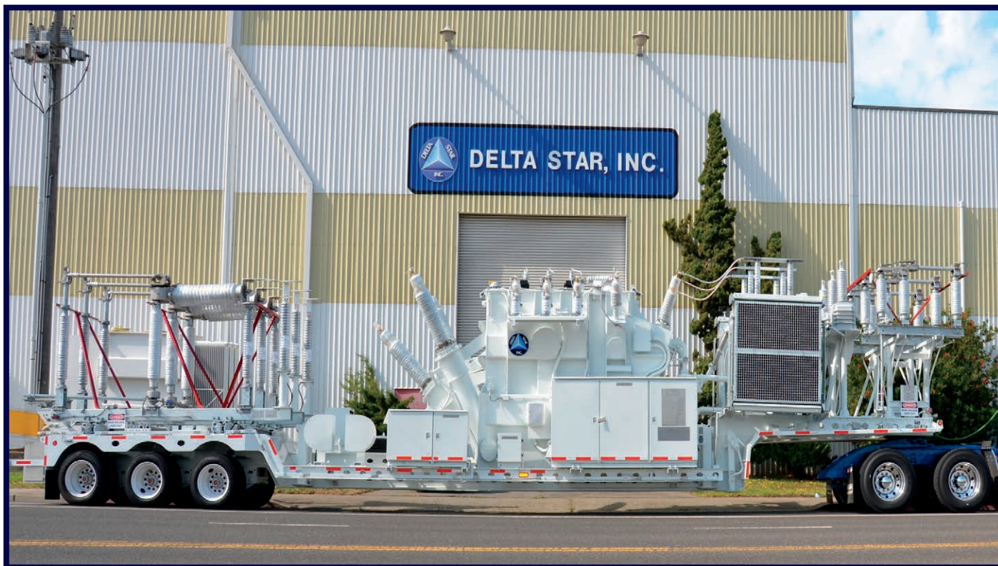
(50 MVA, 138 kV - 69 kV) 2017 | 56' | 129,000 lbs. Customer Region: WEST
