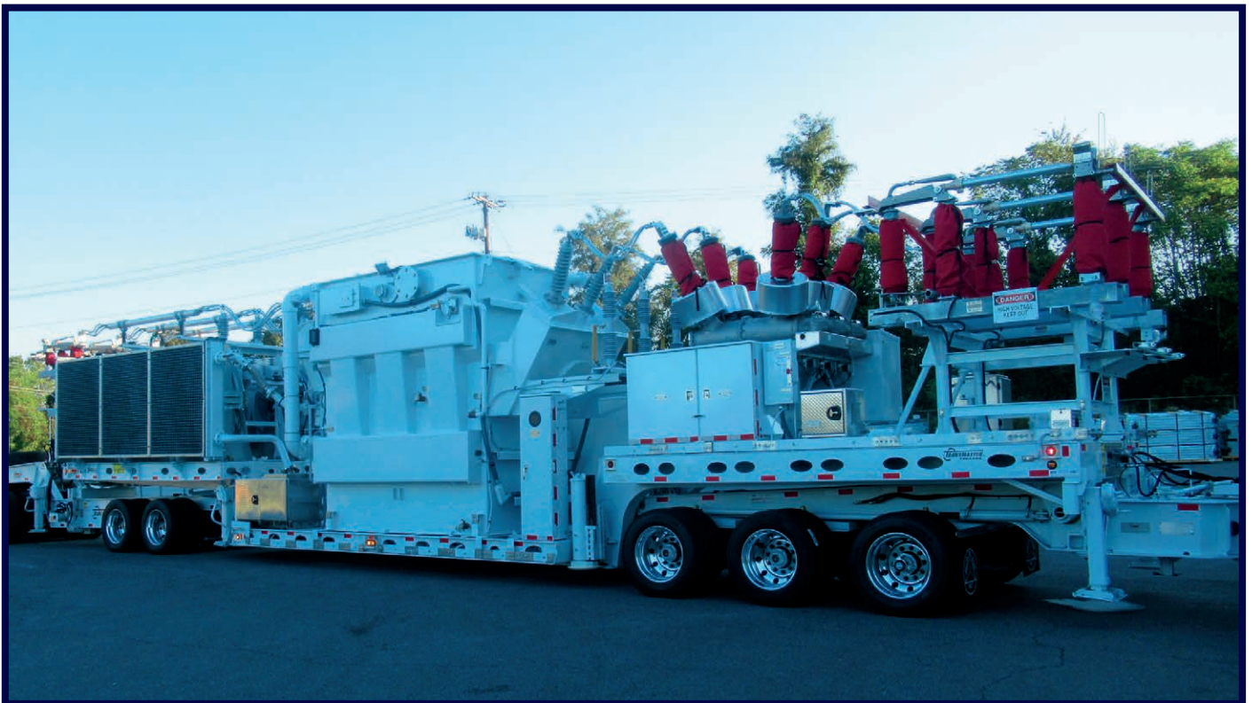
(60 MVA, 69 kV - 13.8 kV, LTC) 2019 | 84' | 179,000 lbs. HV SF6 Breaker Customer Region: ATLANTIC
