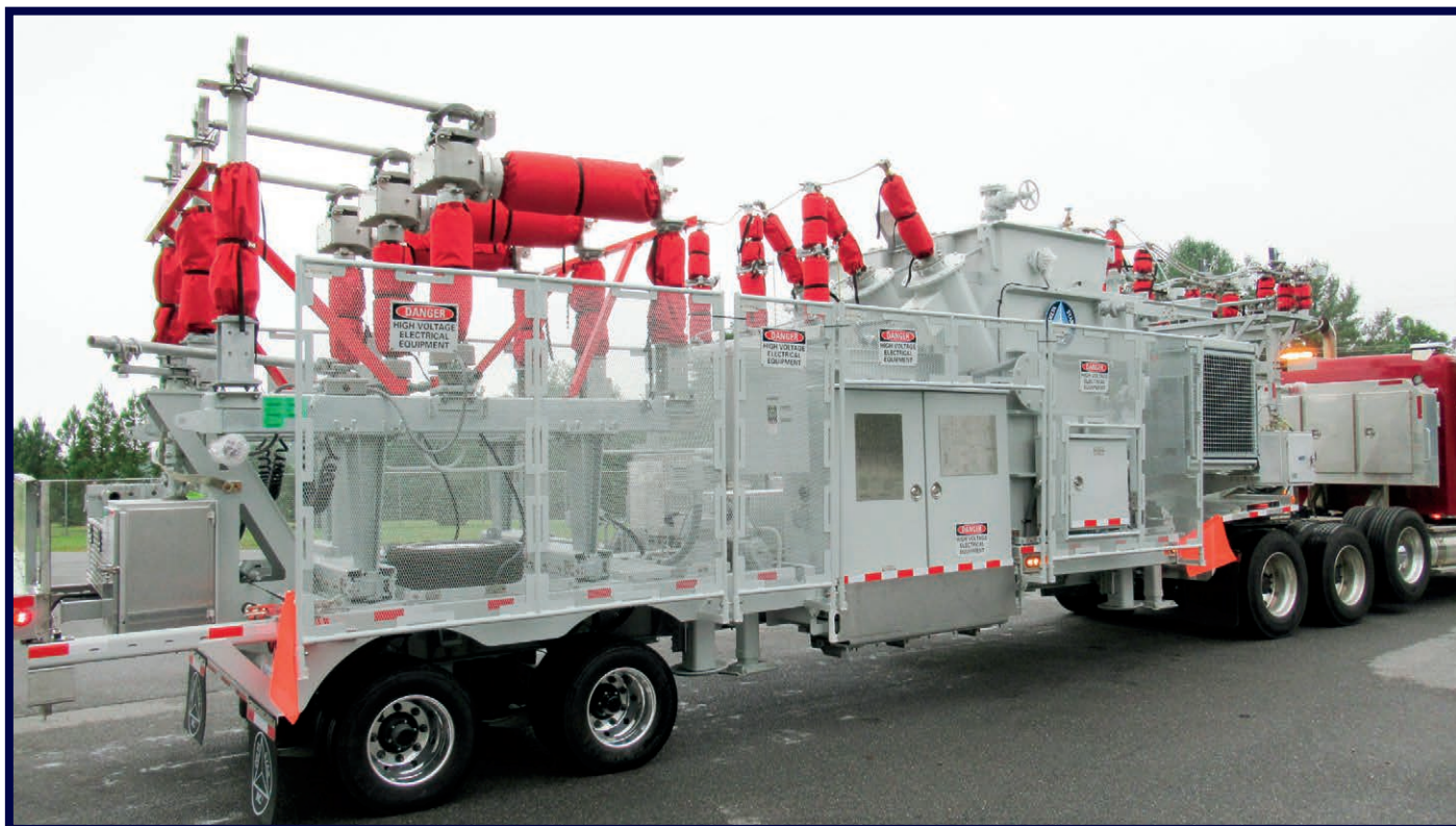
(7 MVA, 69 kV - 12.47 kV) 2018 | 36' | 85,000 lbs. HV Circuit Switcher Customer Region: WESTERN CANADA
