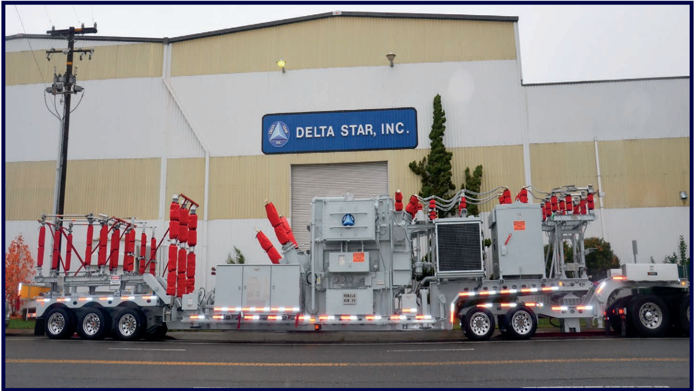
(25 MVA, 115 kV - 24.94 kV, LTC) 2017 | 70'-5" | 171,000 lbs. Customer Region: WEST
