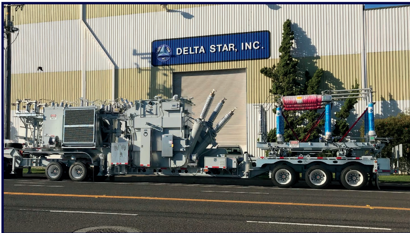
(28 MVA, 115 kV - 24.94 kV) 2019 | 62'-5" | 125,000 lbs. Customer Region: SOUTHEAST
