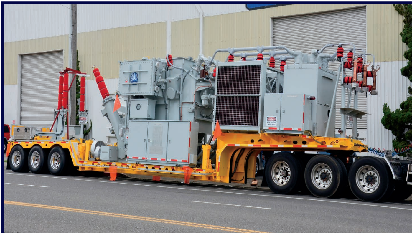
(40 MVA, 115 kV - 13.2 kV, LTC) 2014 | 50' | 128,000 lbs. Customer Region: ATLANTIC
