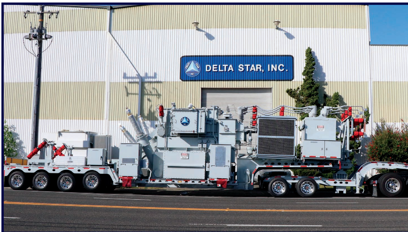
(25 MVA, 117 kV - 34.5 kV, LTC) 2019 | 69'-10 1/4" | 175,000 lbs. Customer Region: WEST
