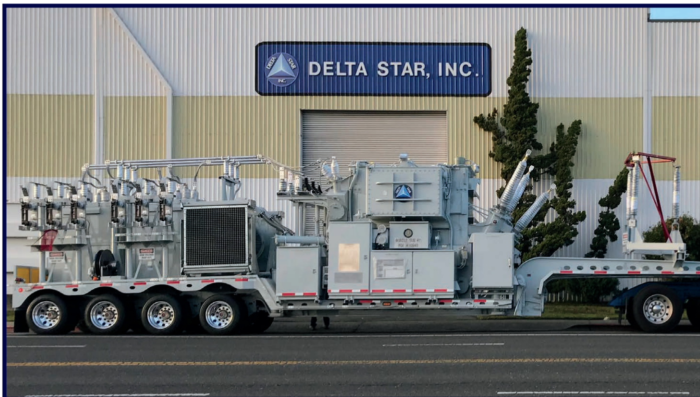
(27 MVA, 120 kV - 13.2 kV, LTC) 2017 | 54' | 140,000 lbs. Customer Region: WEST
