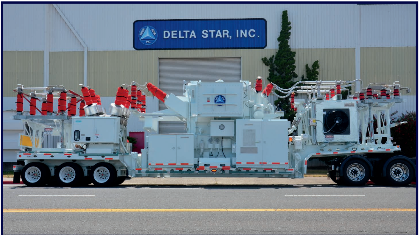
(20 MVA, 69 kV - 4.37 kV, LTC) 2015 | 46' | 120,000 lbs. Customer Region: ATLANTIC
