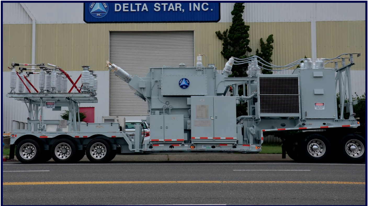
(30 MVA, 69 kV - 26.4 kV) 2014 | 42' | 113,000 lbs. Customer Region: SOUTHEAST
