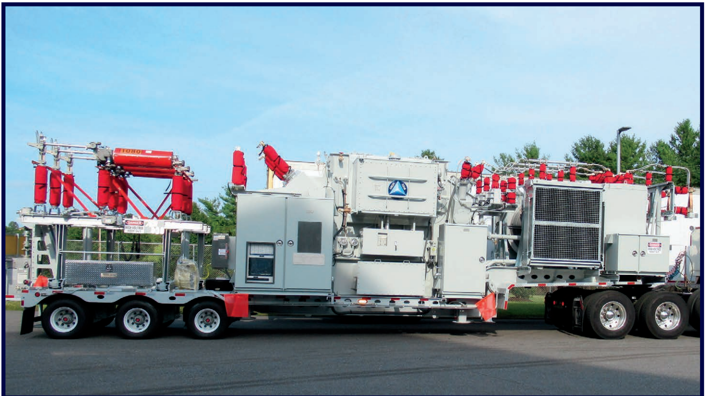
(25 MVA, 69 kV - 26.18 kV, LTC) 2017 | 42' | 112,000 lbs. LV Vacuum Breaker and HV Circuit Switcher Customer Region: MIDWEST
