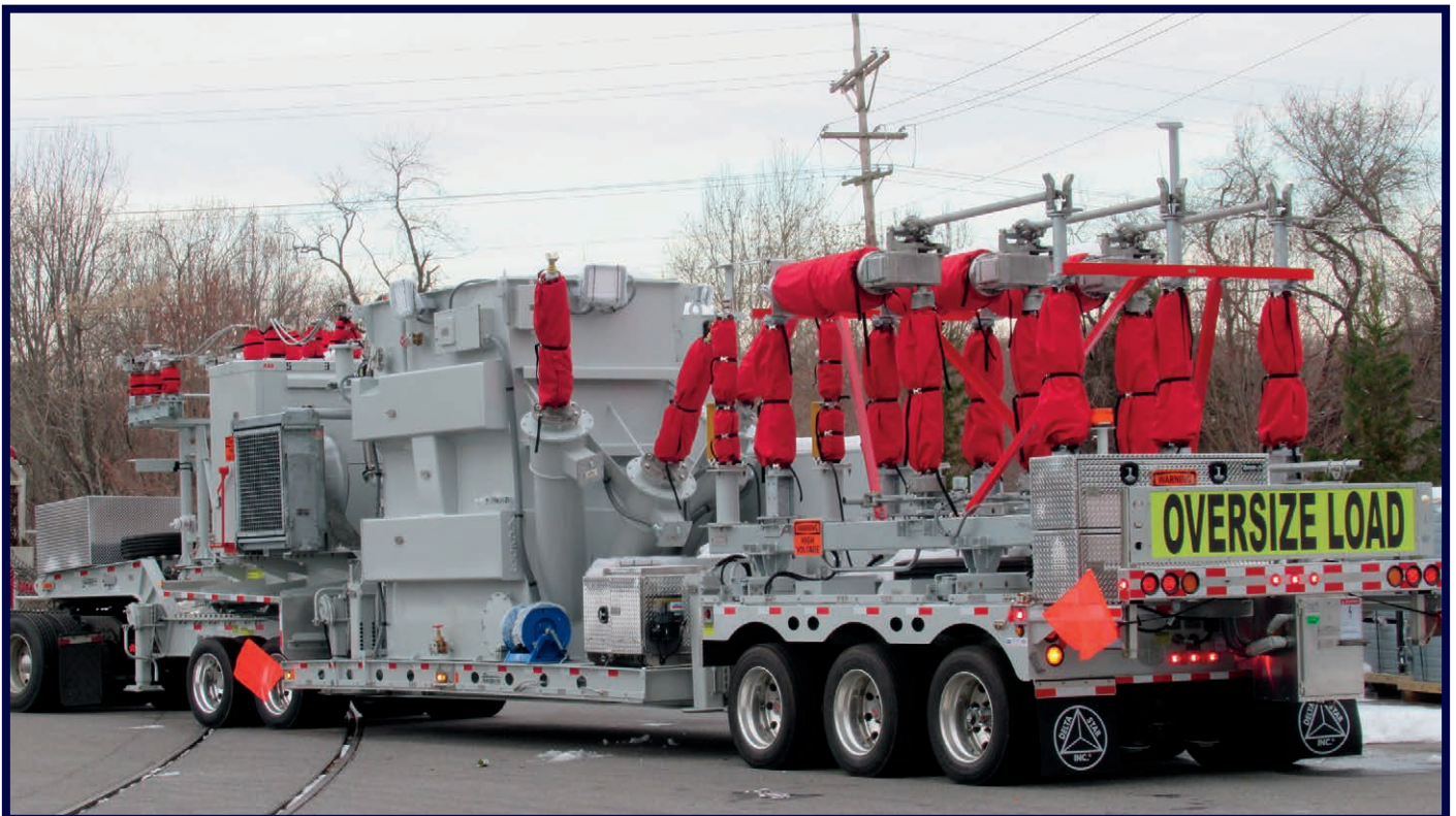
(15 MVA, 115 kV - 13.09 kV, LTC) 2018 | 62'-6" | 127,000 lbs. LV Vacuum Breaker and HV Circuit Switcher Customer Region: SOUTHEAST
