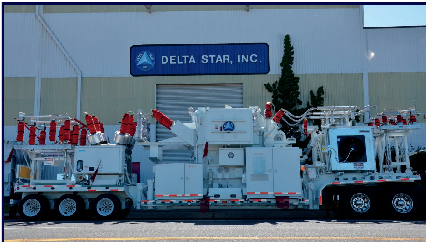
(20 MVA, 69 kV - 4.37 kV, LTC) 2015 | 46' | 120,000 lbs. Customer Region: ATLANTIC
