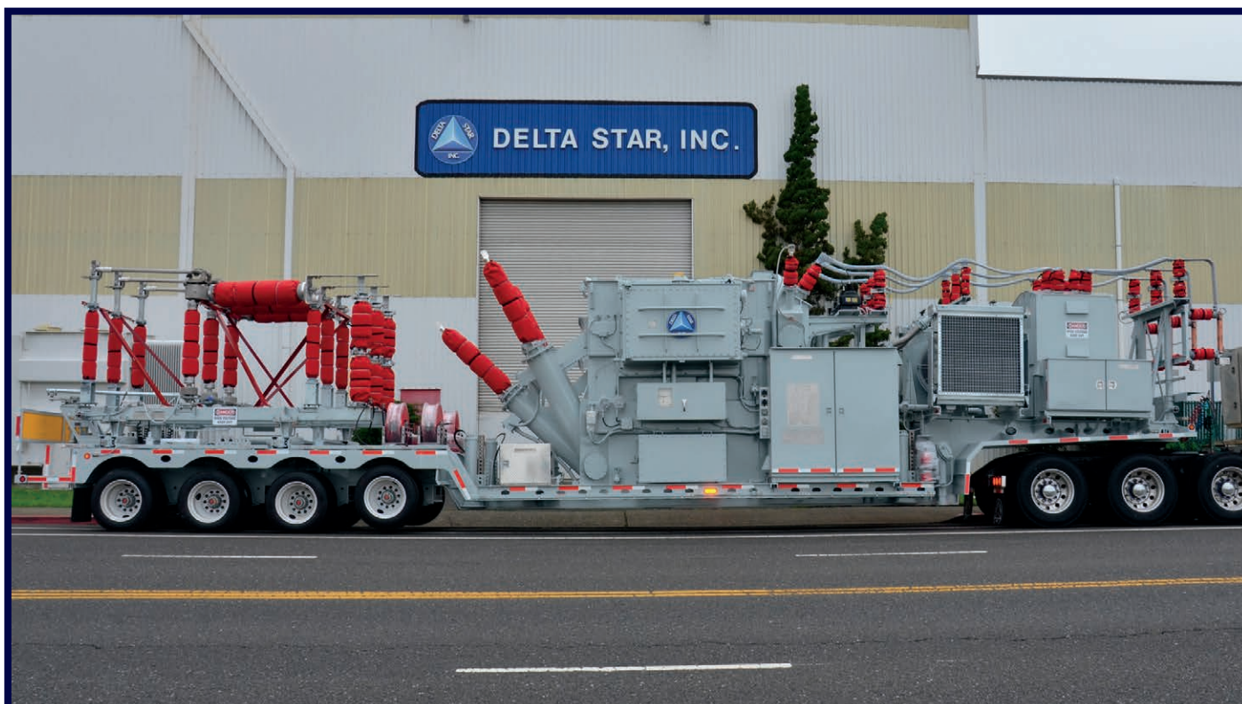
(20 MVA, 115 kV - 26.4 kV, LTC) 2015 | 54' | 112,000 lbs. Customer Region: MIDWEST
