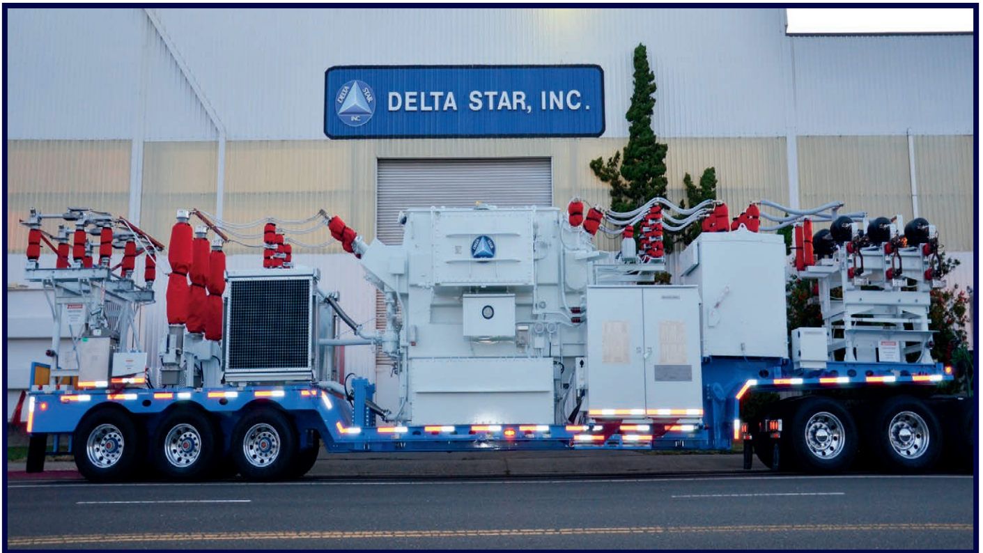
(20 MVA, 46 kV - 13.09 kV, LTC) 2017 | 50' | 128,000 lbs. Customer Region: MIDWEST
