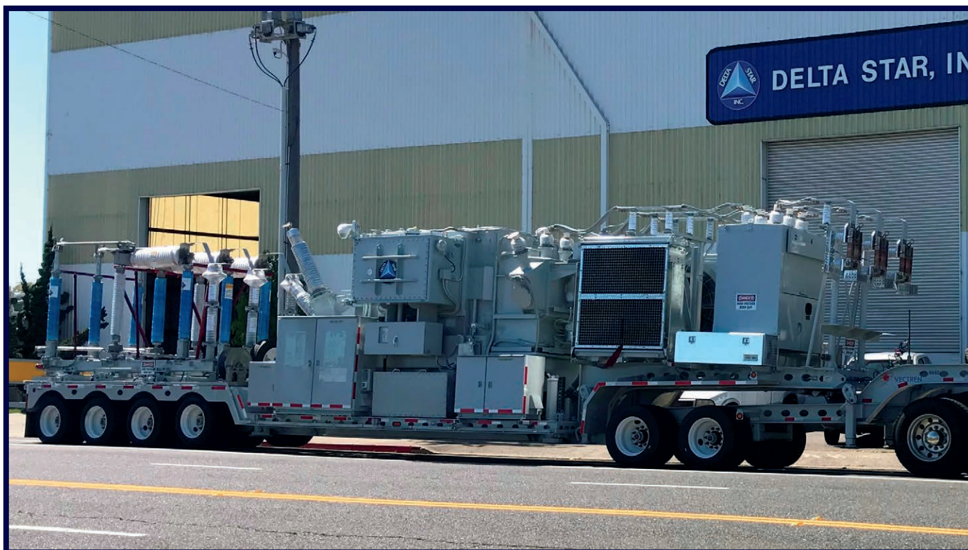
(25 MVA, 138 kV - 13.09 kV, LTC) 2019 | 60' | 221,900 lbs. Customer Region: MIDWEST
