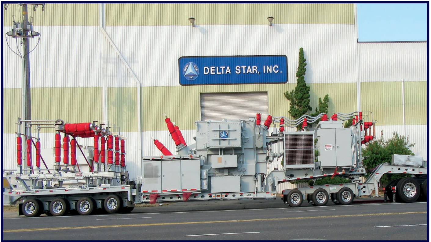
(30 MVA, 138 kV - 26.18 kV, LTC) 2015 | 68'-5" | 168,000 lbs. Customer Region: WEST
