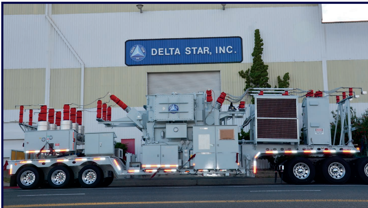
(37 MVA, 33.5 kV - 13.2 kV, LTC) 2015 | 50' | 128,000 lbs. Customer Region: ATLANTIC
