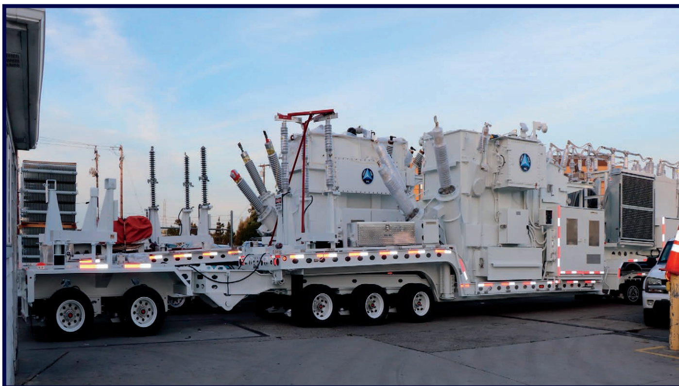
(30 MVA, 138 kV - 37.74 kV, LTC) 2018 | 50' | 130,000 lbs. Customer Region: MIDWEST
