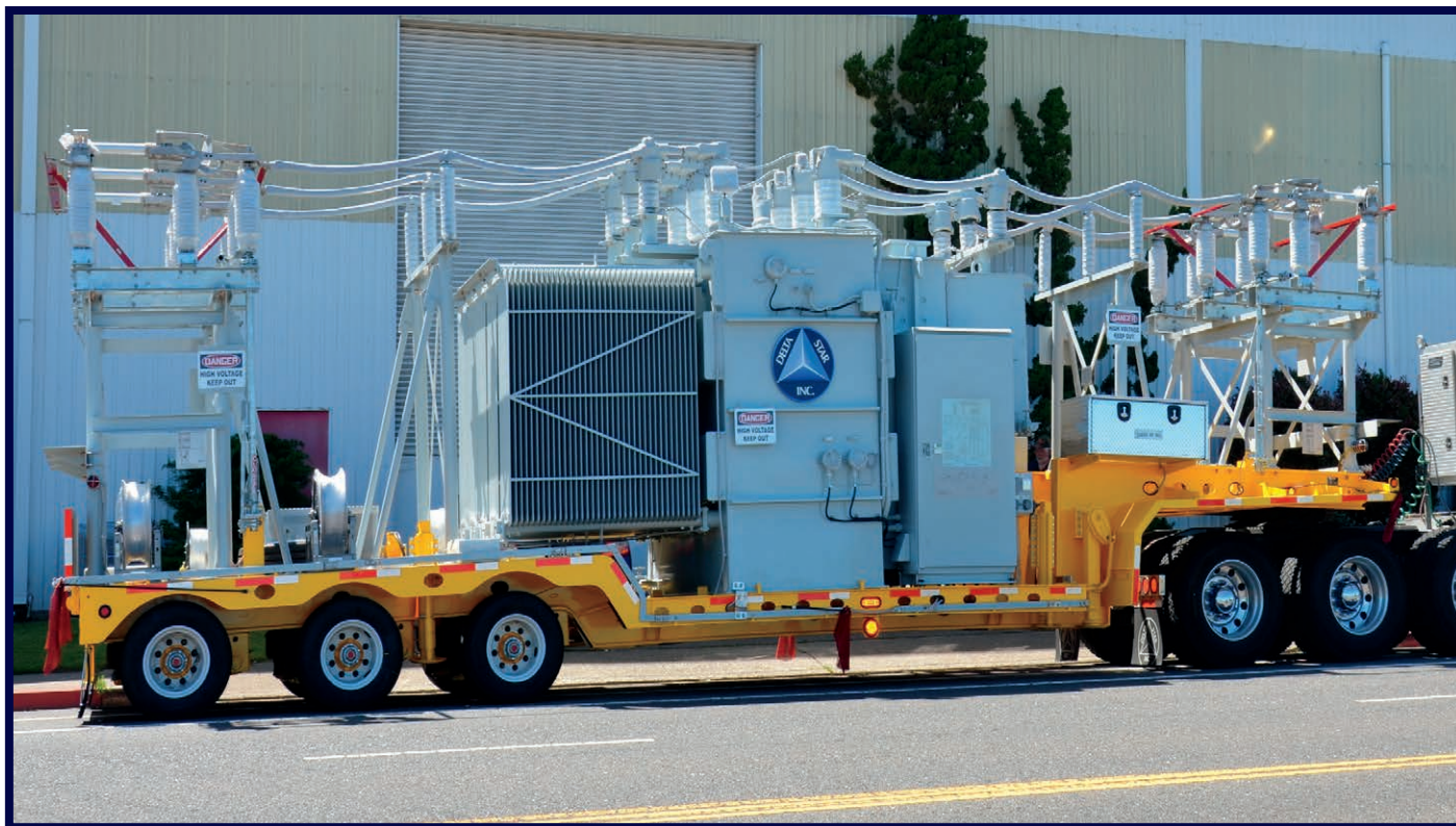
(4 MVA, 34.5 kV - 34.5 kV, LTC) 2016 | 42' | 112,000 lbs. Customer Region: ATLANTIC
