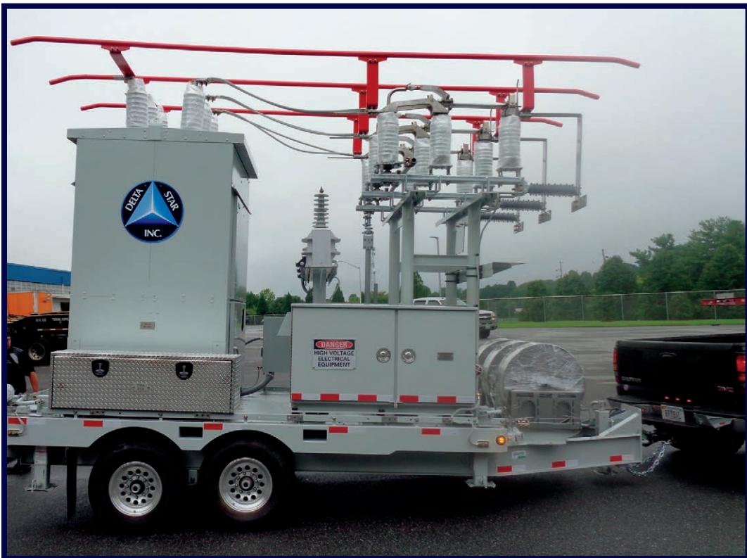
Mobile Circuit Switcher Trailer Customer Region: ATLANTIC
