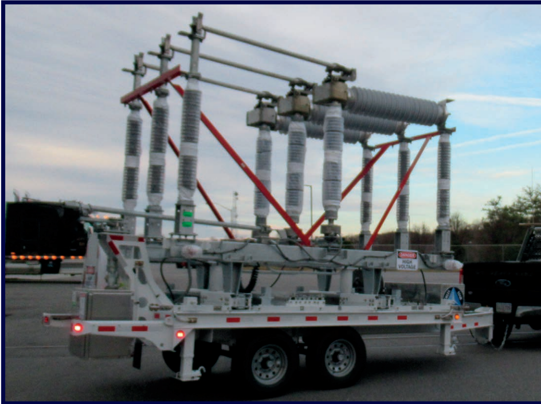
Mobile Circuit Switcher Trailer Customer Region: SOUTHWEST
