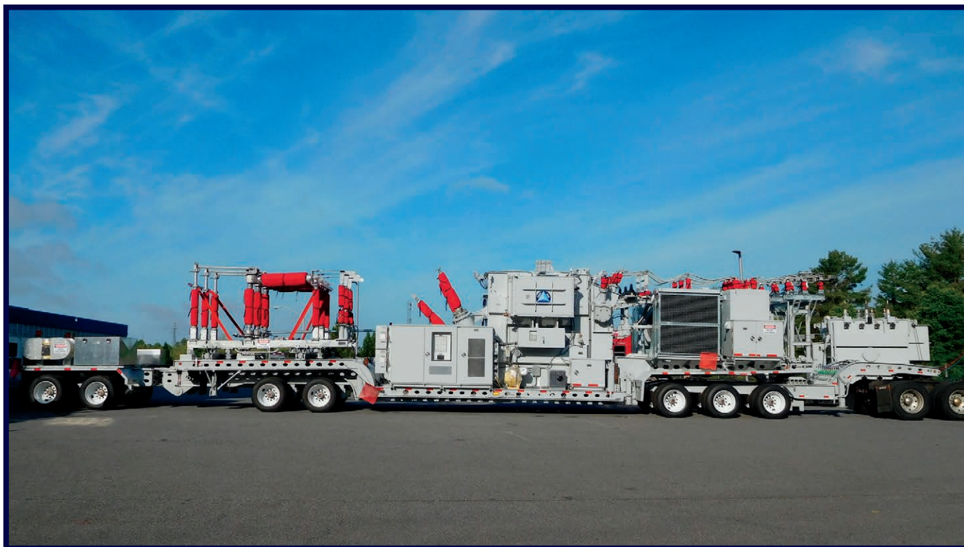
(35 MVA, 115 kV - 13.09 kV, LTC) 2018 | 52'-7" | 161,000 lbs. LV Vacuum Breaker and HV Circuit Switcher Customer Region: SOUTHEAST
