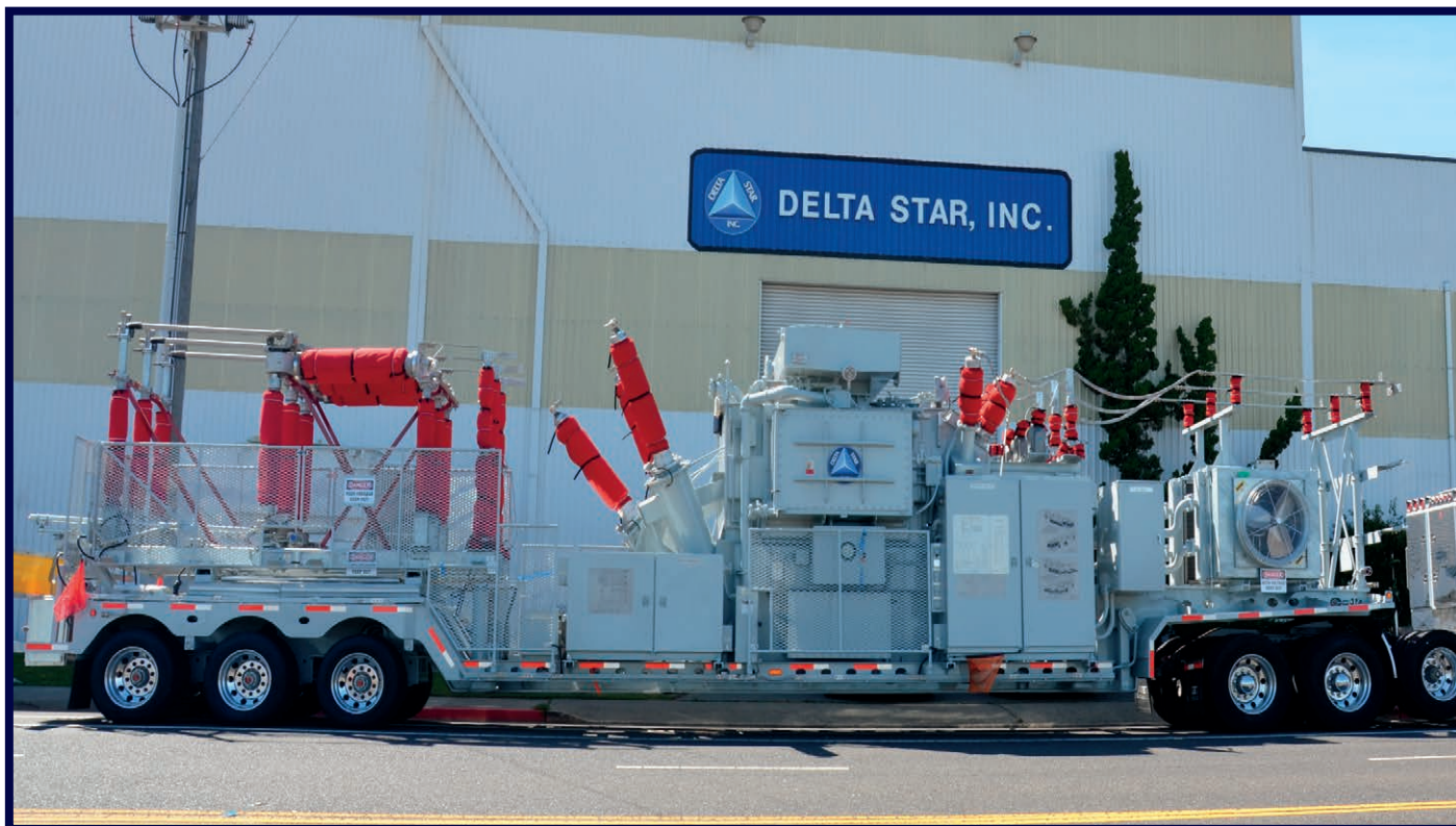
(15 MVA, 138 kV - 25.2 kV, LTC) 2015 | 60' | 150,000 lbs. Customer Region: EASTERN CANADA
