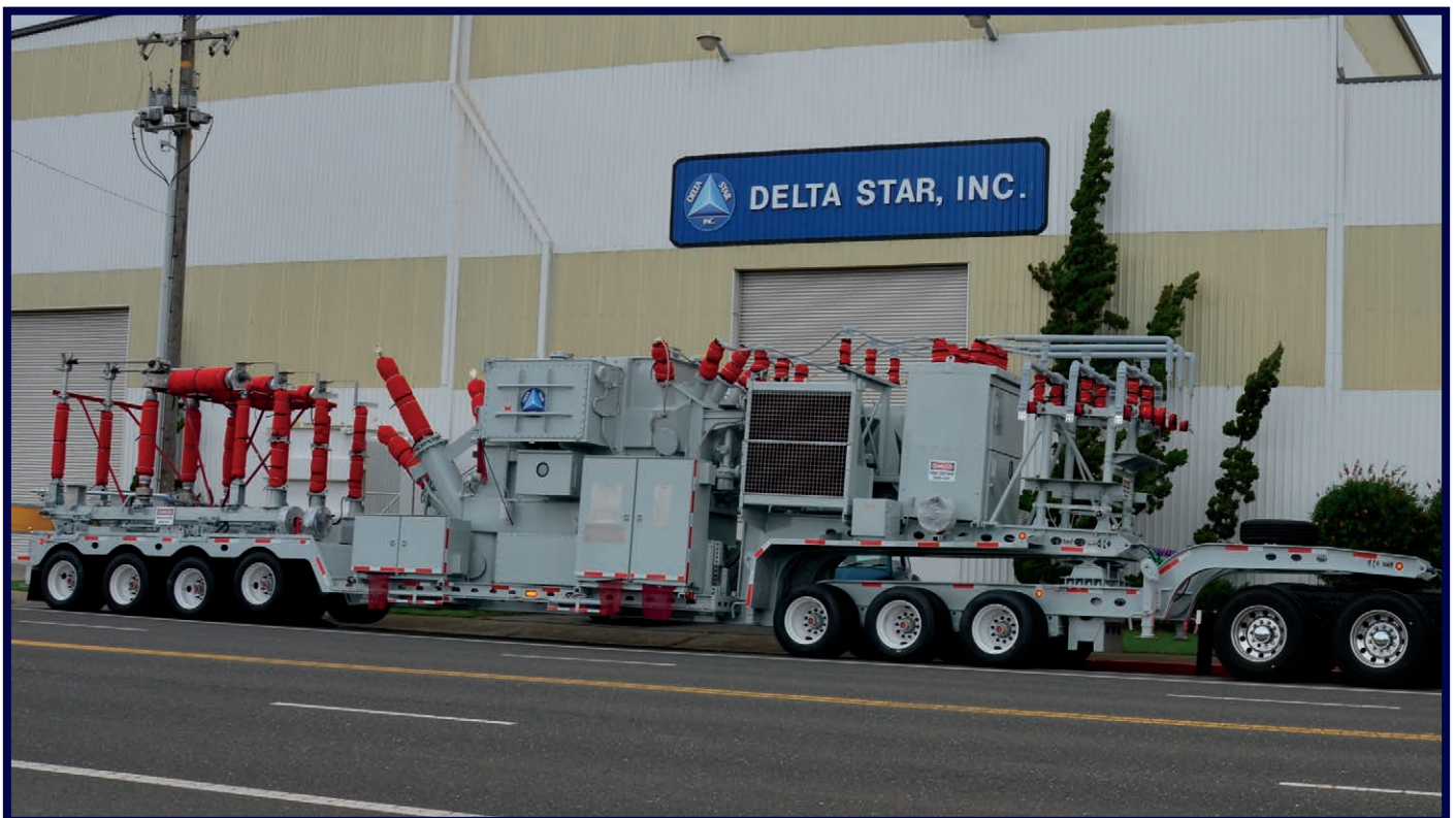
(28 MVA, 138 kV - 26.4 kV, LTC) 2014 | 68'-5" | 174,000 lbs. Customer Region: WEST
