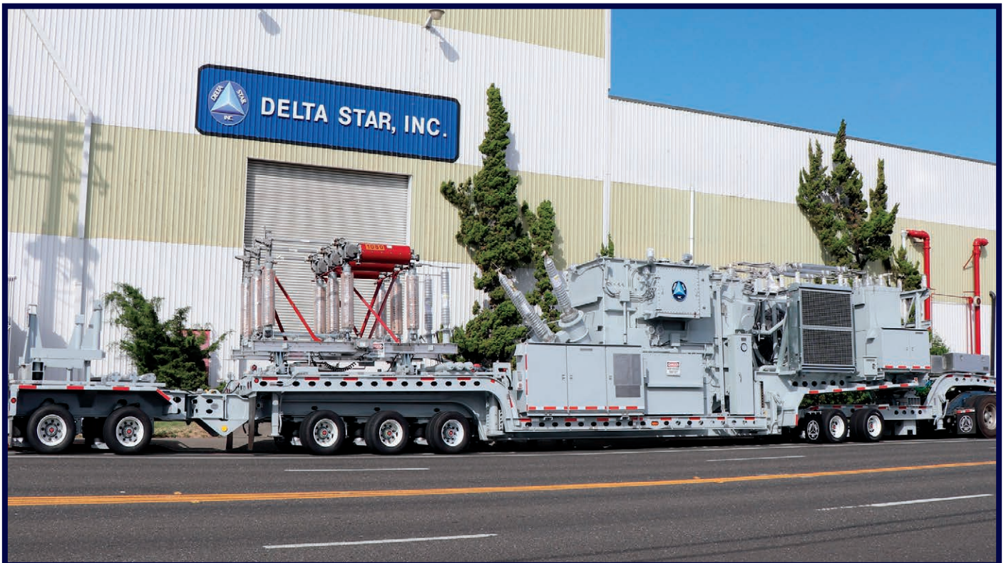
(33 MVA, 115 kV - 14.4 kV, LTC) 2019 | 82' | 180,000 lbs. Customer Region: SOUTHEAST
