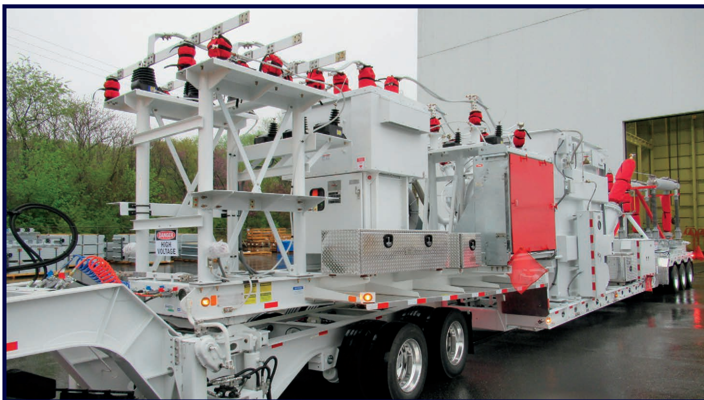
(25 MVA, 138 kV - 13.09 kV, LTC) 2018 | 71'-5" | 141,000 lbs. LV Vacuum Breaker and HV Circuit Switcher Customer Region: MIDWEST
