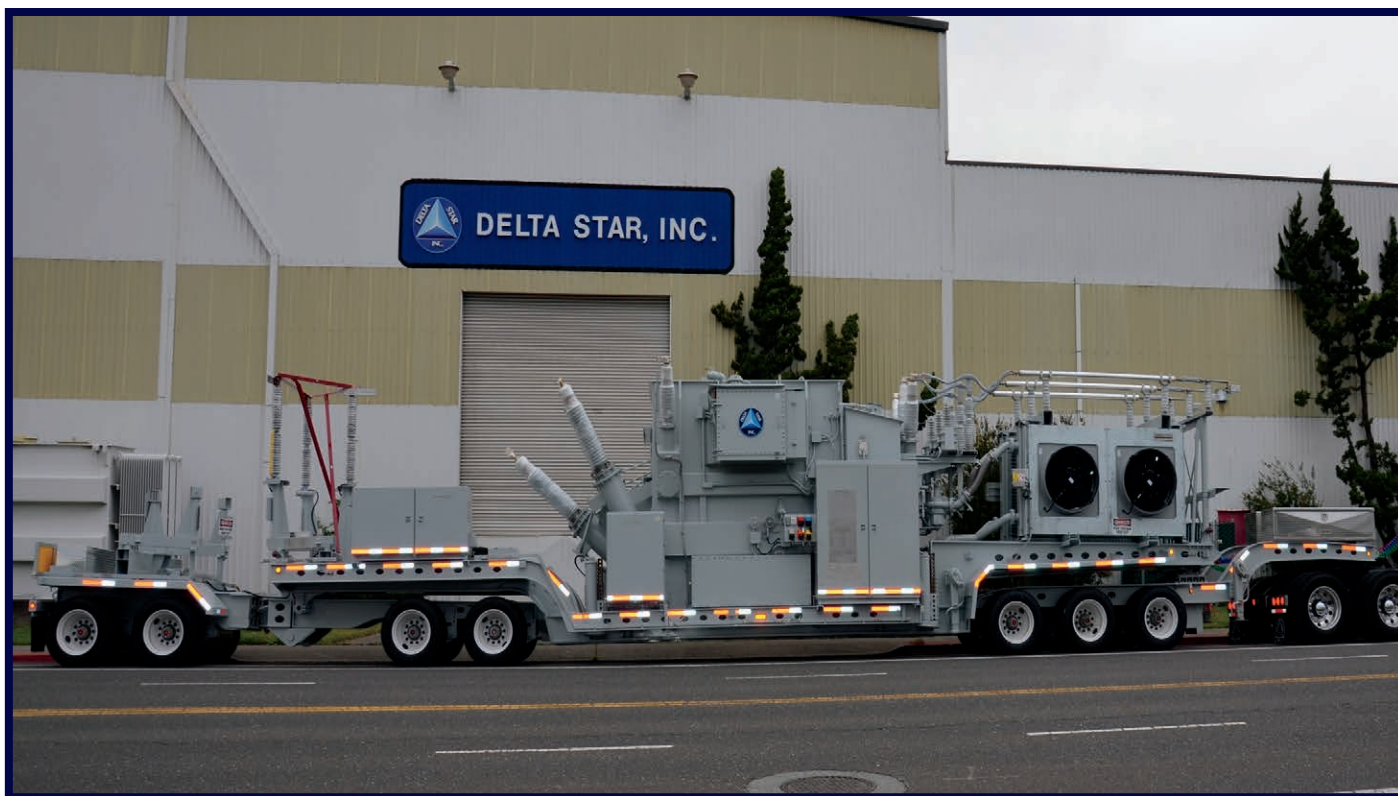
(50 MVA, 141 kV - 37.5 kV, LTC) 2017 | 59' | 164,000 lbs. Customer Region: WEST
