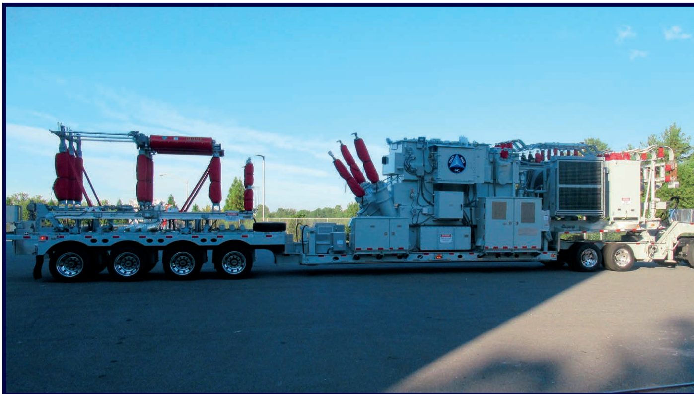
(25 MVA, 138 kV - 13.2 kV, LTC) 2019 | 70'-5" | 158,000 lbs. LV Vacuum Breaker and HV Circuit Switcher Customer Region: WEST
